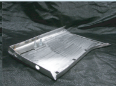
Left and right side tail pans 074951-505L and -505R
