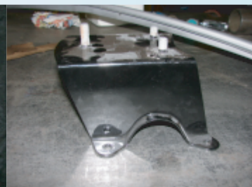
Outer spare tire mounting bracket 074950-521
