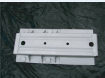
Inner spare tire mounting bracket 074950-520
